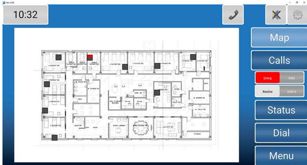
When a call is placed from a station, the top portion of the icon will change color depending on the type of call being placed — blue for code blue shown below. These icons can also be used to direct dial a station.
