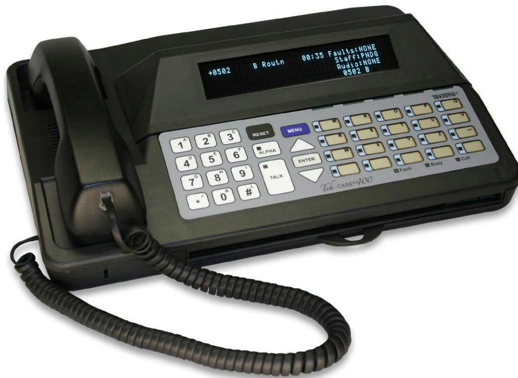
On the home screen of the NC401VFD Master Station, press **Menu** twice on the keyboard to get to the **Main Menu**. Scroll through with the up and down arrows and press **Enter** to get to the different menu options. Below is the tree-view navigation chart of different options under the **Main Menu**. Press **Menu** to get back to the **Home** screen.
