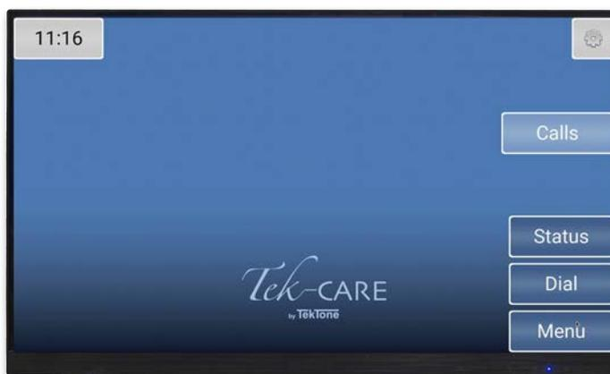
The NC404TS Tek-CARE Master Station provides all of the features of the NC403TS, but adds two-way voice communication capability between patients and staff. Calls are automatically sorted by priority and duration. The highest priority calls will be displayed first.
