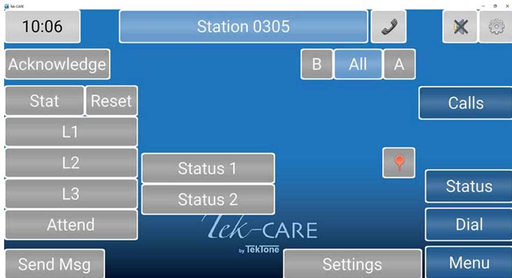
A **Stat** call can be used as a staff emergency. Touch **Stat** if there is an emergency for the patient in the room with that station. Stat can only be reset at either the station itself, the NC402TS, NC404TS, NC415G3, or on the NC404 sidecar. To clear this option at the master station, select **Stat**, touch **Reset**, then press the **RESET** button on the sidecar.
