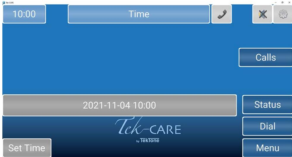
To change the system time or date, touch **Set Time** in the lower left corner of the screen. On the next window that appears, enter the date and time in YYYY-MM-DD HH:MM 24-hour format.
