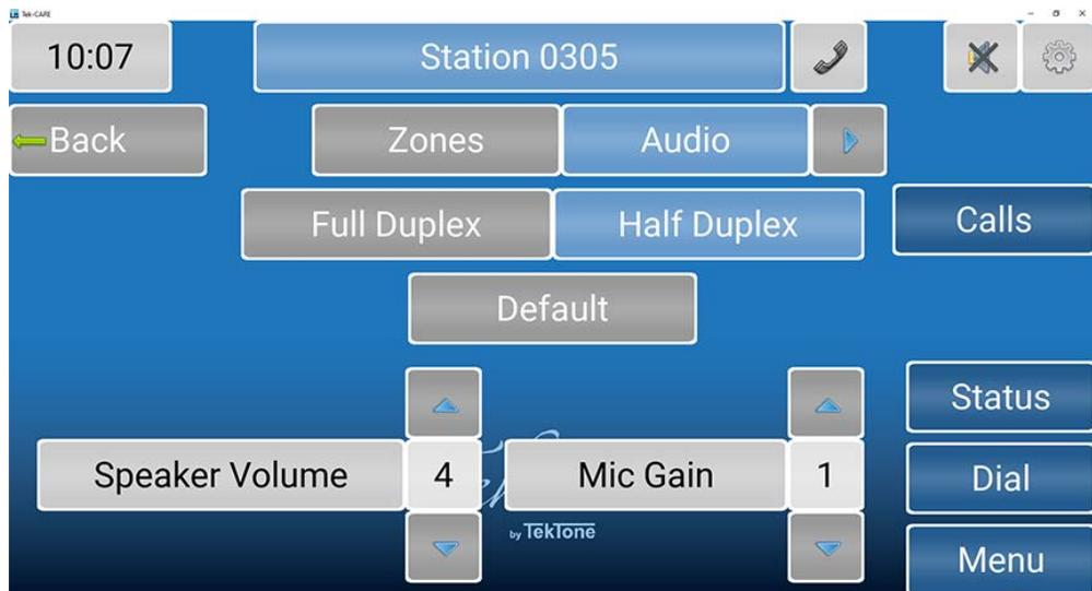
Choose either **Full Duplex** or **Half Duplex**. **Full Duplex** enables simultaneous audio to and from the station (like a telephone - talk and listen simultaneously). **Half Duplex** only allows audio to work from one station at a time (like a radio - push to talk, release to listen).
