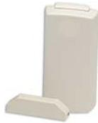
**SF520ES/UL Door/Window Egress Transmitter:** This transmitter is used to monitor door and window activity. It may be used as either NO (Normally Open) or NC (Normally Closed) to allow use in a variety of applications. Alarms are either automatically reset when the device returns to a normal state or when calls are acknowledged by staff, depending on system programming.
