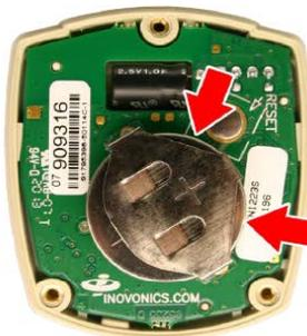
**Figure 10 - SF501ES Battery Orientation**
