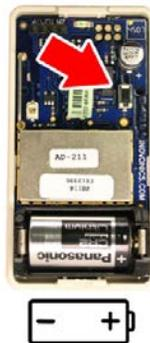
**Figure 15 - Open SF520ES/UL, Figure 16 - SF520ES/UL, SF525ES/UL SF525/2ES/UL, SF527ES/UL Battery Orientation**
