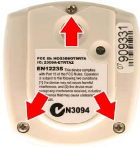
**Figure 9 - SF501ES Battery Removal**
