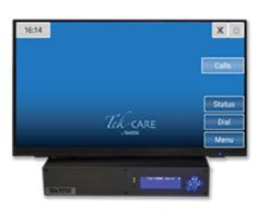
life-safety standards. The Tek-CARE Appliance Server can simultaneously connect to any current TekTone nurse call system, plus a variety of foreign systems-such as fire alarm and security systems.
