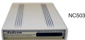
**The NC503 Central Monitoring Modem** is connected to the Tek-CARE Appliance Server via a standard straight serial cable, and is connected to a telephone wall jack using a standard 6-position/2-wire telephone cable. It includes the auto dialer, a straight serial cable, a power adapter with cord, and a telephone cable.
