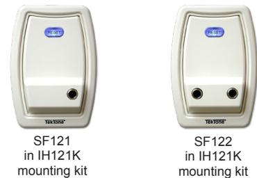
The **SF121 Single Patient Station** includes an illuminated reset button, a ¼" call cord jack, and a call assurance LED. The **SF122 Dual Patient Station** has two jacks and two call assurance LEDs. The stations are surface mounted using a single-gang or dual-gang mounting kit attached to a standard single-gang ring or single-gang ring and box.
