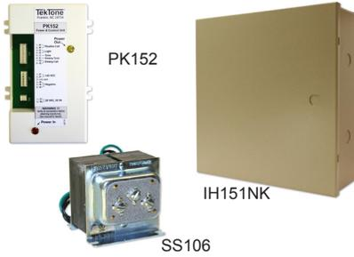
**The IH151NK Power & Control Kit** provides power and control for two states (steady/routine and flashing/emergency) to dome lights when used with an NC50xES-series remote receiver. The kit includes a PK152 Power & Control Unit and an SS106 Class 2 Transformer installed in an IH151N junction box. The PK152 uses pigtail connections. Knockouts are included on all sides (except the lid) to allow the connection of electrical conduit from any direction.
