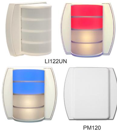
The **LI122UN Room Controller with Dome Light** provides 6 connection points for patient stations, 2-button pull-cord stations, and a duty station; plus visual indication of calls via slide switches to manually select the two dome colors as White/Red or White/Blue and tone of the White color as warm White or cool White. The **PM120 Room Controller** provides the same 6 connection points in locations where a corridor dome light is not needed.
