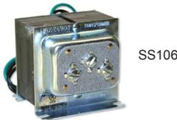
**The SS106 Class 2 Transformer** offers a compact, easy-to-install low voltage AC power source for use with TekTone® intercom systems. The transformer is UL® Listed and will safely take itself offline when overheated. It is designed for easy installation in a standard 1/2" knockout or for surface installation, and may be used in either plastic or metal boxes.
