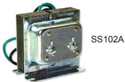
**SS102A Transformer** offers a compact, easy-to-install low voltage AC power source for use with TekTone® intercom systems. The transformer is Class 2 UL® Listed and will safely take itself offline when overheated. The transformer is constructed for easy installation in a standard 1/2" knockout or for surface installation, and may be used in either plastic or metal boxes.
