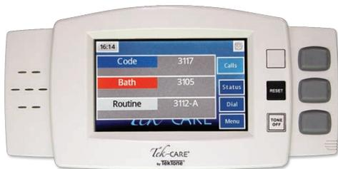
The compact master stations can be either wall- or desk-mounted. The LCD touchscreen lists patient calls by priority in a pleasing display, and calls are annunciated via pleasant call tones to reduce institutional noise. A dome light may be connected directly to the master station to indicate the highest-priority call originating in the master's zones.
