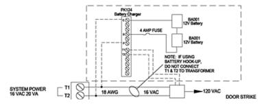
**PK124 TE Diagram** (partial drawing, refer to IL573 for full drawing)
