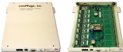
**The NC377-series Voltage Interface** (Paging Interface Adapter) connects switched voltage analog systems (such as Tek-CARE NC200, NC150, NC110) to the Tek-CARE Appliance Server. NC377-series accept 5–50V AC or DC input, and recognize three states: off, steady on, and flashing. The NC377/32 includes 32 inputs; the NC377/64 includes 64 inputs. Up to 9 NC377-series Voltage Interfaces may be connected together to accommodate up to 576 inputs.
