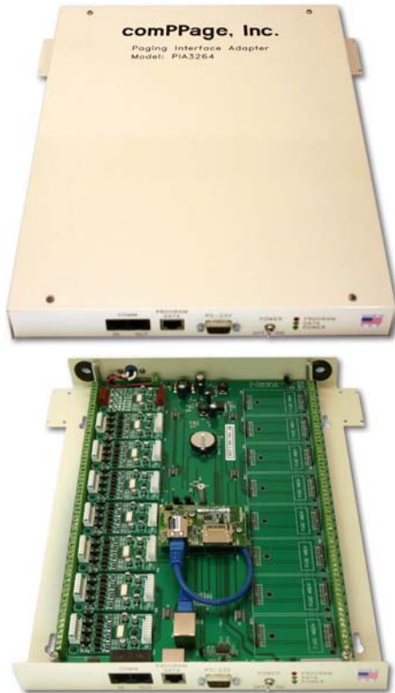
NC377/32 Paging Interface Adapter (exterior & interior)
